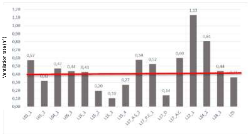
Figure 5. Results of ventilation rates in winter using constant emission method (phase 2)
